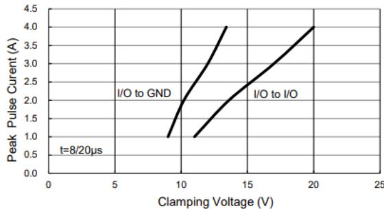
**Fig 6 Transmission Line Pulsing (TLP) Measurement**
